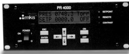
The PR4000 is a versatile 4½-place digital LCD display/power supply unit available in both one and two-channel versions. Both units have two fully configurable relays for set point monitoring, RS-232 digital interfaces with optional RS-485 and IEEE-488 interfaces, 16-bit analog output, and auto zero capability. The PR4000 can be used with Type 622, 623, 624, 625, 626, 627, and 628 capacitance manometers.
